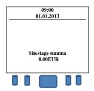
Enter the sum of the transaction as a final sum (for instance customer have to pay 15€, so you insert 1500). Then press a GREEN button (Enter). YELLOW button is for correcting the sum. RED is for a transaction cancellation.
