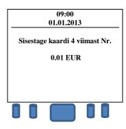
Enter 4 last customer's card numbers and press the GREEN button. Terminal connects to the bank.
